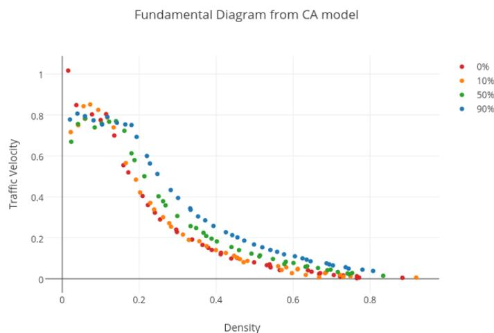
Figure 4: density and velocity data from our cellular automata model.
