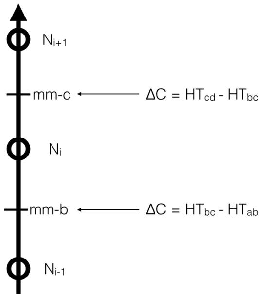
Figure 2: Schematic of  $i$ th road segment as a circular node. Here mm- $x$  refers to mile-marker  $x$ , and  $\Delta C$  keeps track of the cars that have entered or exited the road between nodes.
