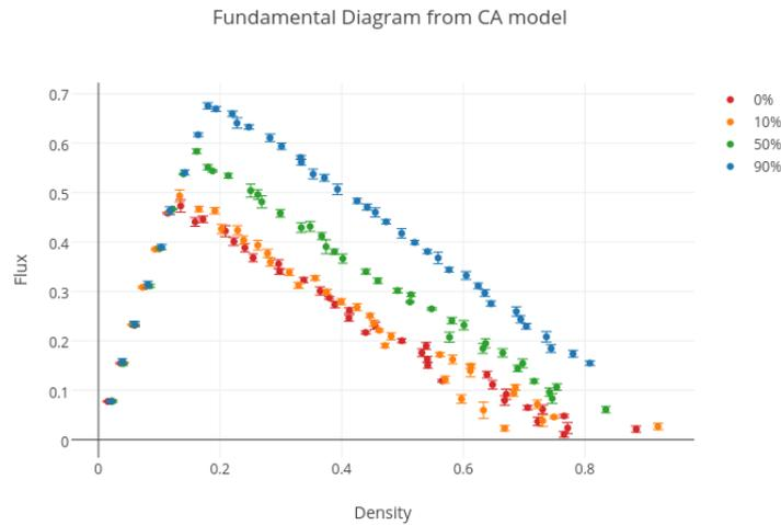
Figure 3: density and traffic flux data from our cellular automata model.
